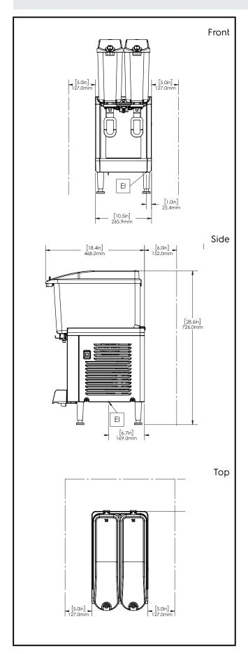
Simplicity Bubblers Chilled Beverage Dispensers 2x9 L, agitator model with locking lid
